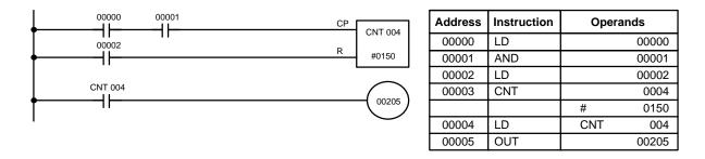
Here, 00000 can be used to control when CNT is operative and 00001 can be used as the bit whose OFF to ON changes are being counted.
